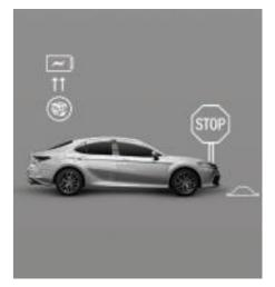
**REGENERATIVE BRAKING** The motor generator recovers the kinetic energy from braking which recharges the hybrid battery.
