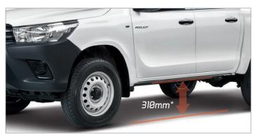
GROUND CLEARANCE - Keep Operations Going and Deliver No Matter What the Road Condition. 195mm (Hilux 4x2J) and 310mm (Hilux 4x4J)
