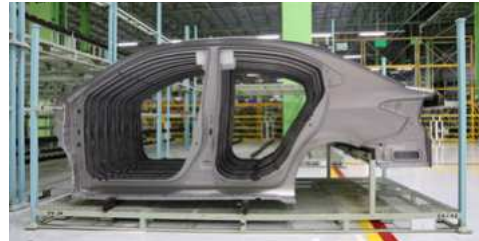
Vios side member produced at TMP’s A Zero-class press stamping shop
