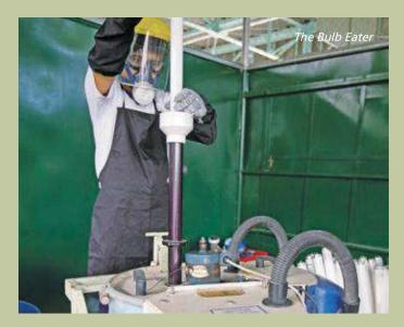
TMP also utilizes the bulb-eater, equipment designed to capture the mercury vapor content of busted fluorescent lamps. The Bulb Eater's 3-stage filtration system can capture 99.99% of airborne particles, including mercury vapor.
